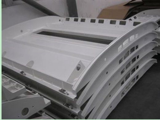
SMC bus HVAC housing
