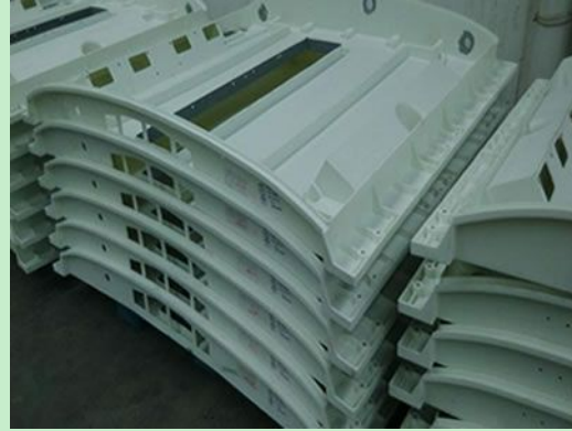
D-LFT molding bus climate housing
